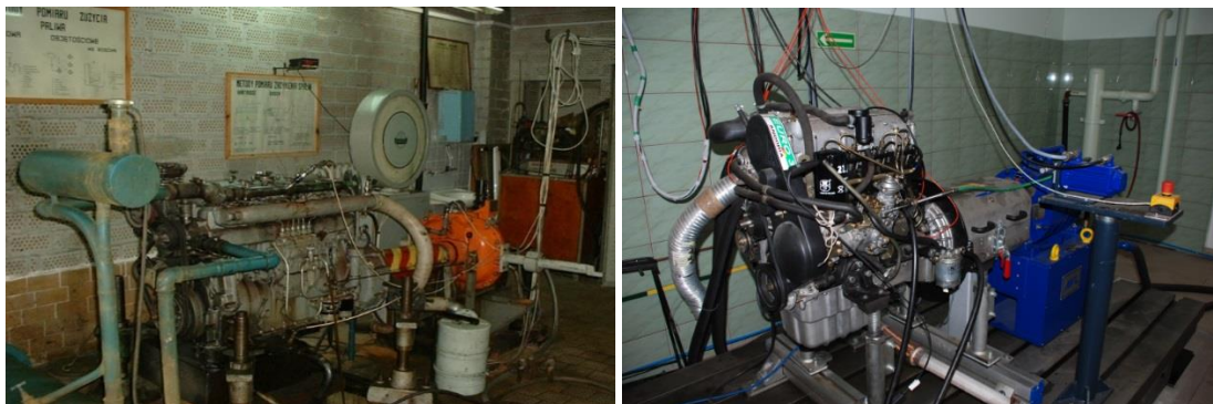
Braking stands for testing engines with fuel pre-treatment
