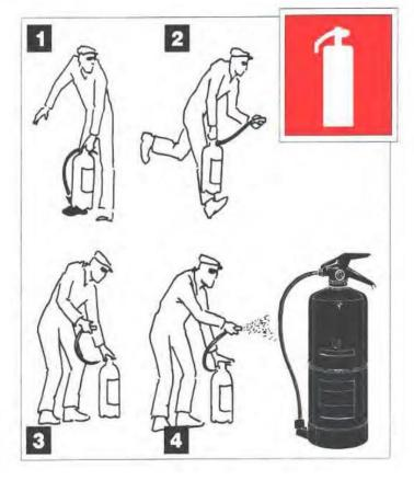
**Foam extinguisher** - a cylinder fitted with a secured handle that, when squeezed, activates the valve or piercer opening a high-pressure gas. The foam-producing agent is discharged through a nozzle or a hose with a nozzle in which the chemical is aerated and foamed. The agent is expelled by high-pressure inert gas, nitrogen or CO2, or foam production through a chemical reaction. Due to its siphon type construction, the extinguisher works properly only in the vertical position.
