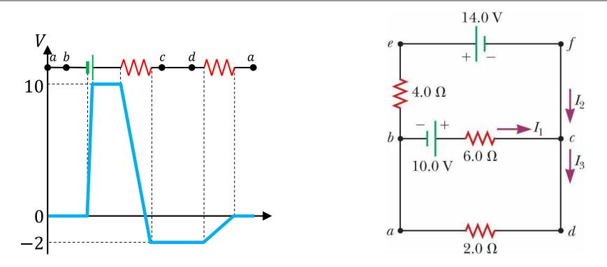
Task: plot potential diagram for befcb path.
