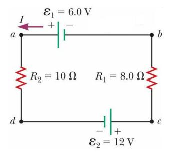
Find the currents  $I_1$ ,  $I_2$ , and  $I_3$  in the circuit shown in the figure.
