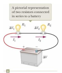
A circuit diagram showing the two resistors connected in series to a battery  $\begin{array}{c} R_1 & b \\ \hline \Delta V_1 & \Delta V_2 \\ \hline I_1 & I_2 \end{array}$
