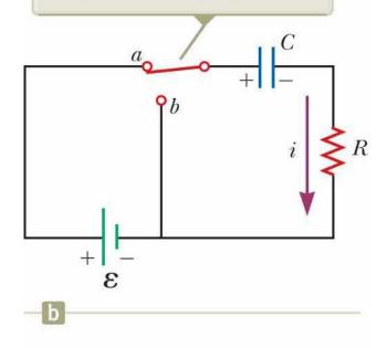
When the switch is thrown to position *b*, the capacitor discharges.
