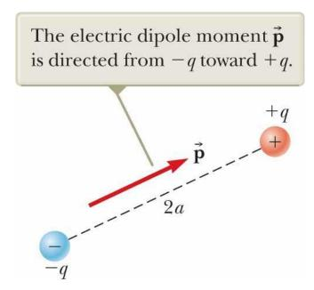
**Electric dipole moment:** vector  $\vec{p}$  directed from -q toward +q along line joining the charges, with magnitude
