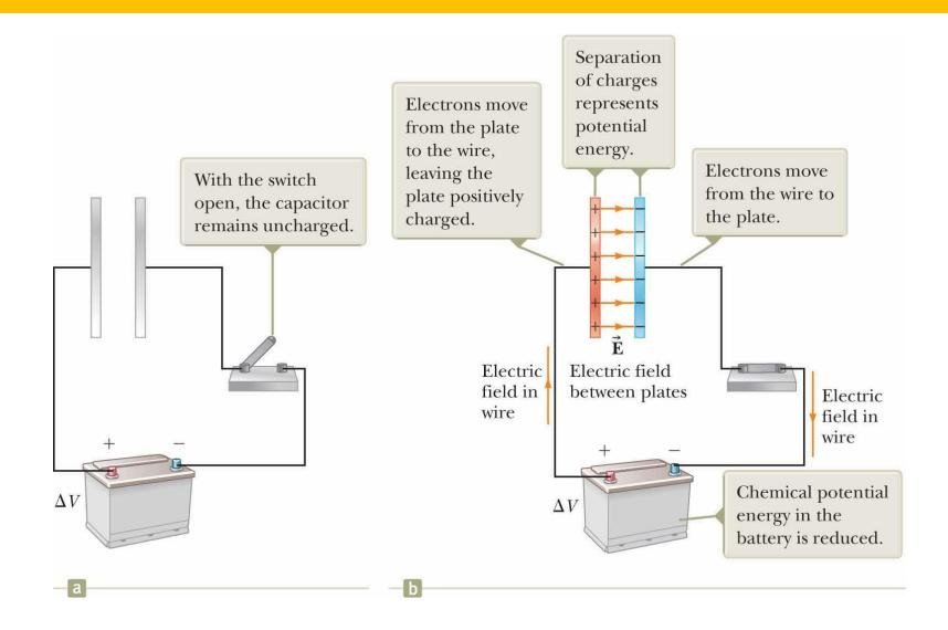
Work necessary to transfer increment of charge dq from plate carrying charge -q to plate carrying charge q (at higher electric potential) is:
