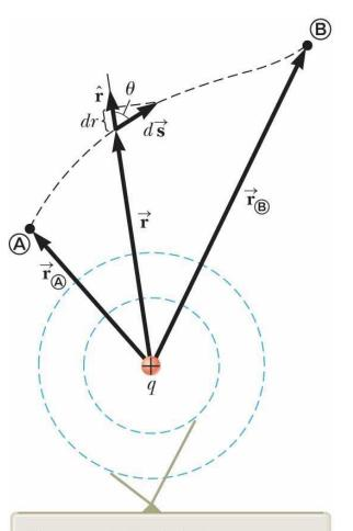
The two dashed circles represent intersections of spherical equipotential surfaces with the page.
