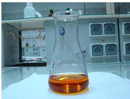
Fig. 6. Sample after adding the tested water, ready for titration
