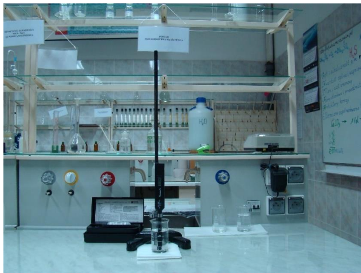
Fig. 7. Laboratory workplace for determination of conductivity
