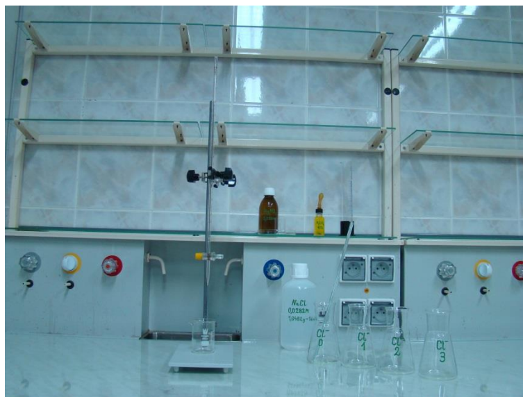
Fig. 2. Laboratory workplace for determination of chloride ions by Mohr's method
