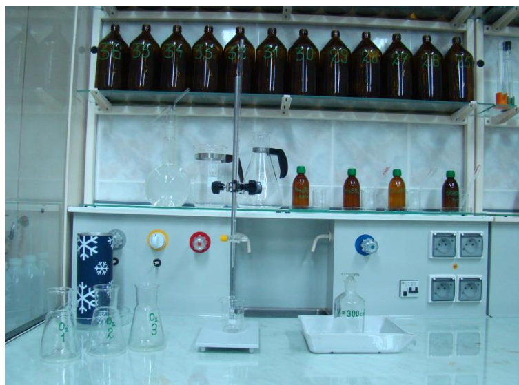
Fig. 2. Laboratory stand for the determination of oxygen in water using the Winkler method
