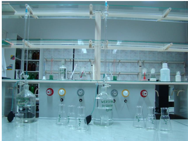
Fig. 1. Laboratory stand for determination of total hardness and calcium hardness
