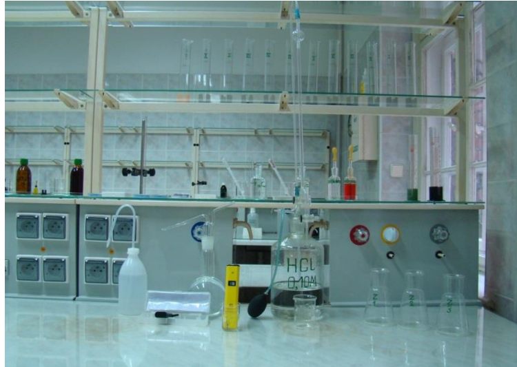
Fig. 3. Laboratory workplace for determination of pH and alkalinity p and m of water
