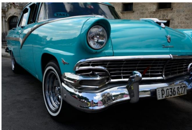
Fig. 6. Chrome-plating of steel parts of classic cars used to give a decorative and protective effect source: https://rhkhydraulics.com/blog/hard-chrome-plating-extending-the-life-of-your-equipment (accessed January, 14, 2022)
