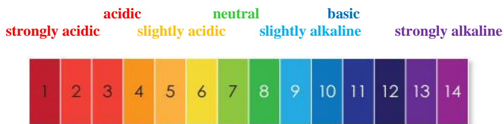
Fig. 1. The ranges of the pH of the solution and the corresponding colours of the universal indicator
