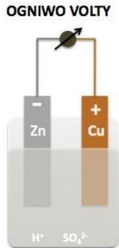
Rys. 4. Schemat ogniwa Volty
