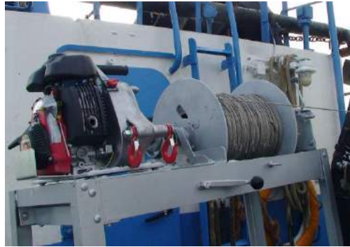
Figure 11. The winch used for closing the sleeve of codend cover.
